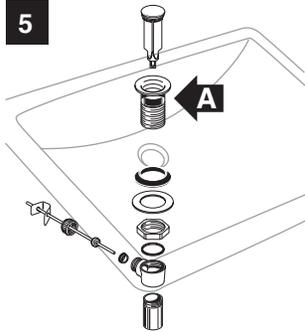
Mount the drain assembly (not included) on the sink, following faucet manufacturer's instructions. Be certain to apply a bead of sealing putty on the underside of the drain (Part "A") in order to ensure a watertight seal between the sink and drain. Remove excess putty after installing drain on sink.
