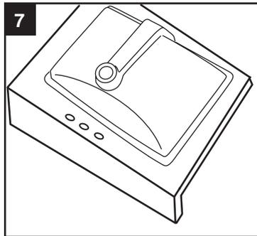
Center bowl over cutout and tighten screws (see 3 or 4) to secure bowl to countertop. Remove excess sealant from inside lip.
