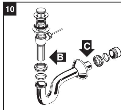
Connect trap to drain assembly hand tight to check alignment. It may be necessary to cut off part of the tailpiece (area "B") or part of the horizontal leg of the trap (area "C"). Secure joints for watertight assembly.
