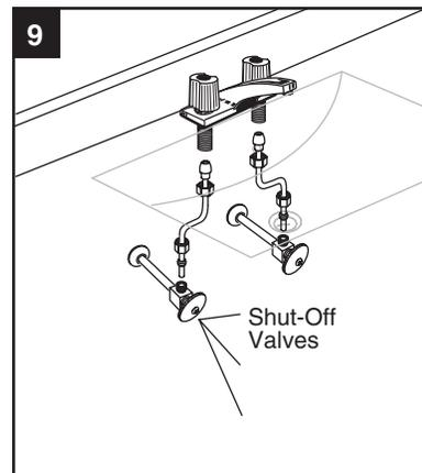
Connect supply line to faucet (finger tight) and carefully bend tubes to engage with the supply shut-off valves. Tighten connections at faucet and shut-off valves for water tight seal.
