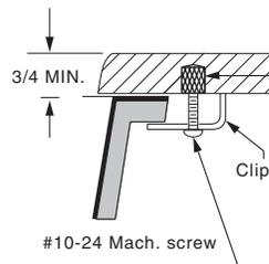
Brass insert, epoxy in place with threaded end exposed. (Epoxy not supplied).
