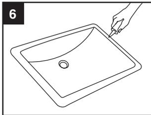
**NOTE:** Do not use adhesives or adhesive sealants. After checking fit and alignment of sink to cut out, apply a bead of silicone adhesive to rim of sink.
