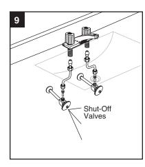
Connect supply line to faucet (finger tight) and carefully bend tubes to engage with the supply shut-off valves. Tighten connections at faucet and shut-off valves for water tight seal.
