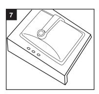
Center bowl over cutout and tighten screws (see 3 or 4) to secure bowl to countertop. Remove excess sealant from inside lip. NOTE: The screws provided should be used on countertops with a minimum 1" thickness. For thinner countertops, use appropriate anchors and fasteners.
