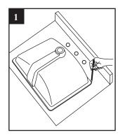
NOTE: To avoid damage to countertop, install sink such that future removal from underneath the countertop is possible. First, make sure the clearance between the backsplash, faucet, fixtures and cabinets are acceptable for the new sink.
