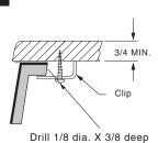
Mark and pre-drill the wood screw holes as located on the enclosed template. Waterproof any exposed areas of wood.
